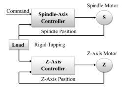
Fig. 2. Synchronous control system
