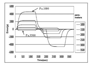
Fig. 8. Waveform showing the synchronization error with parameters  $4065 \sim 4068$
