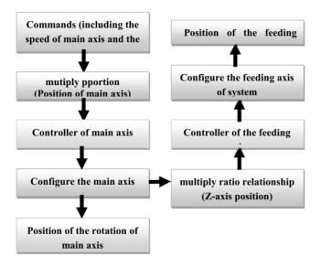
Fig. 1. Control architecture of rigid tapping
